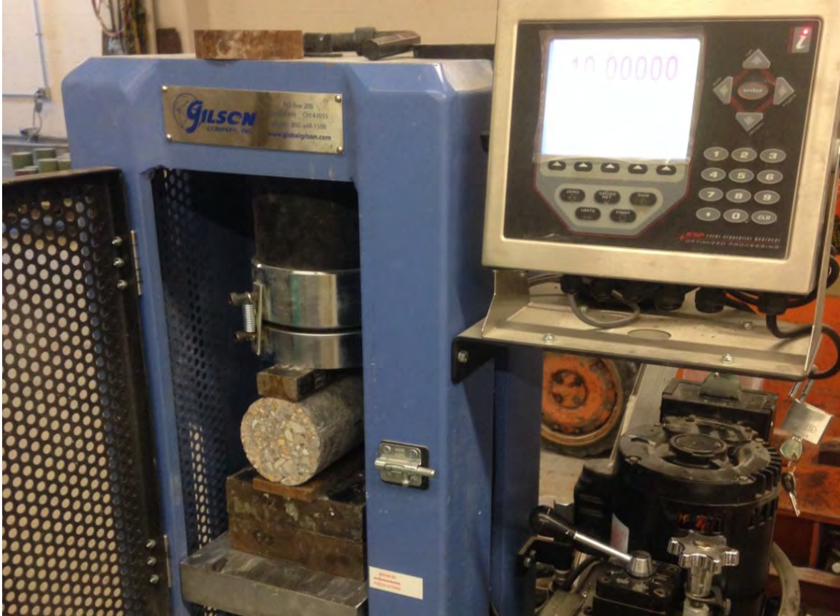
Figure 9- The splitting tensile test setup used in this program
