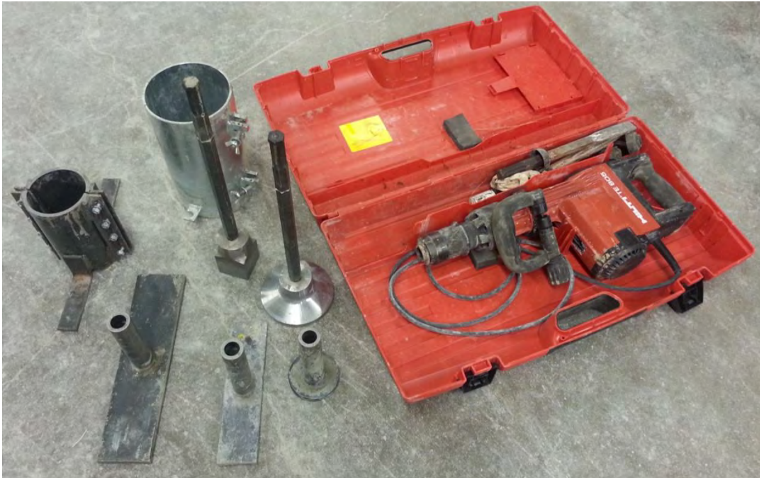
Figure 6- Hammer, rectangular head and circular heads used for sampling RCC
