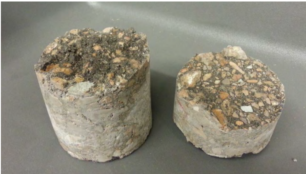
Figure 27- Failure surface in the bond strength test, (left) joint between two lifts, (right) inside the lift
