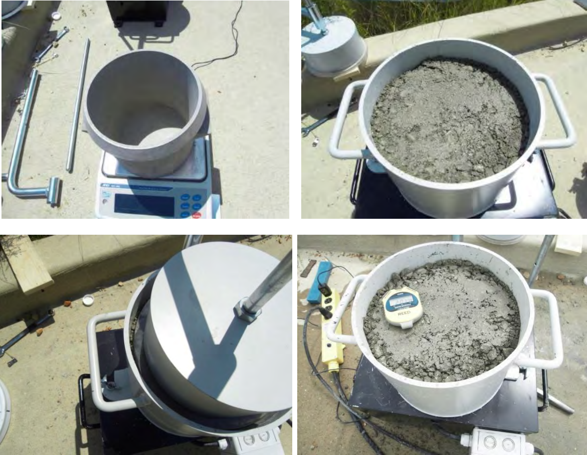
Figure 22- RCC workability test
