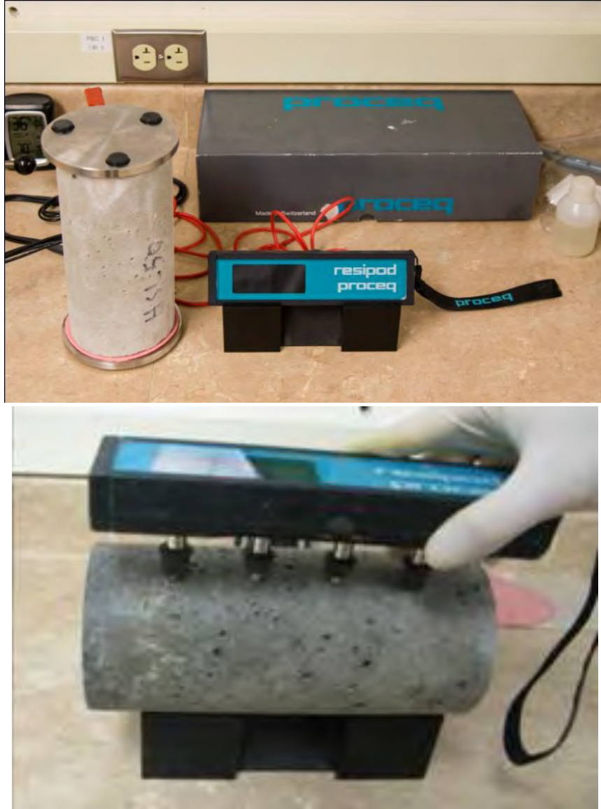
Figure 16- Testing apparatus of surface and bulk resistivity of concrete
