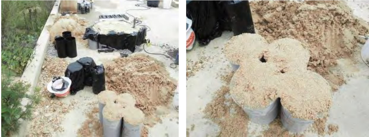
Figure 21- Storage of concrete specimens at the job site
