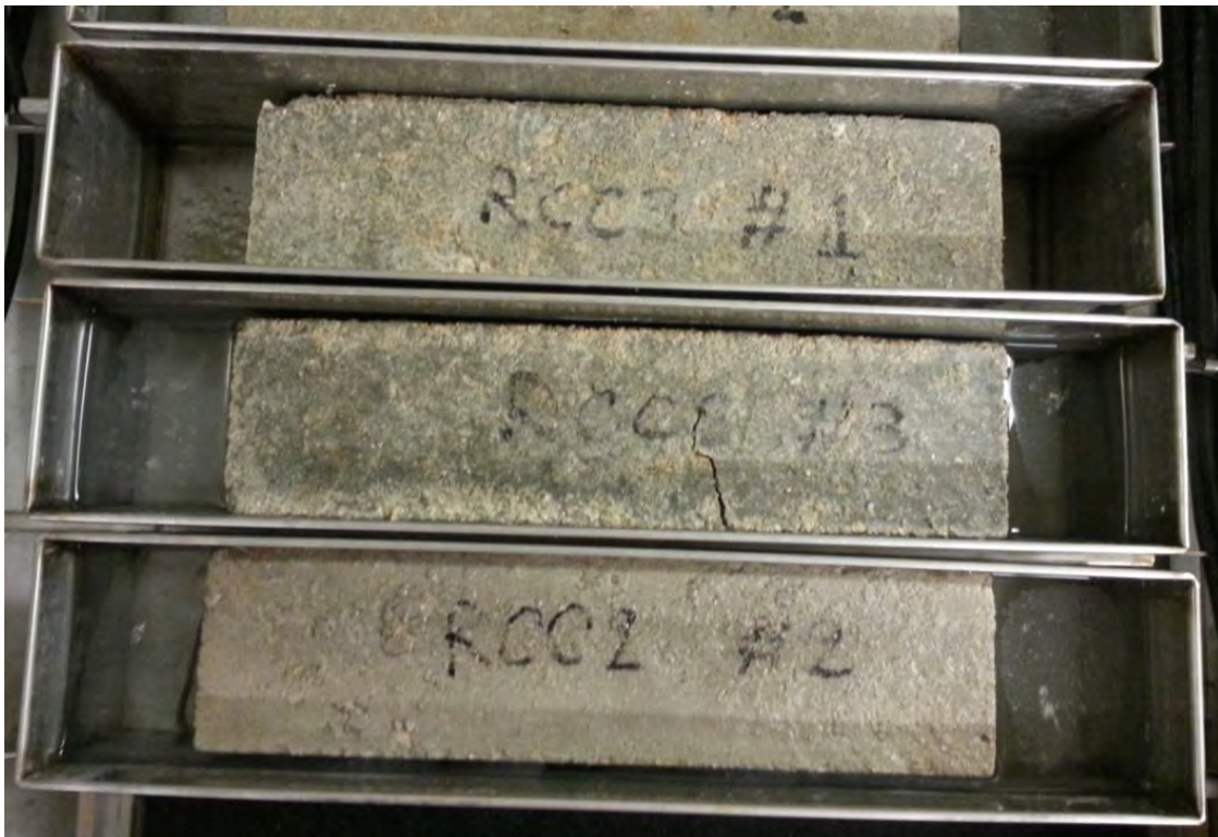
Figure 29- Cast in field RCC specimens after 30 cycles of freezing and thawing
