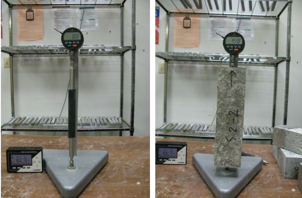
Figure 11- Measurement of drying shrinkage
