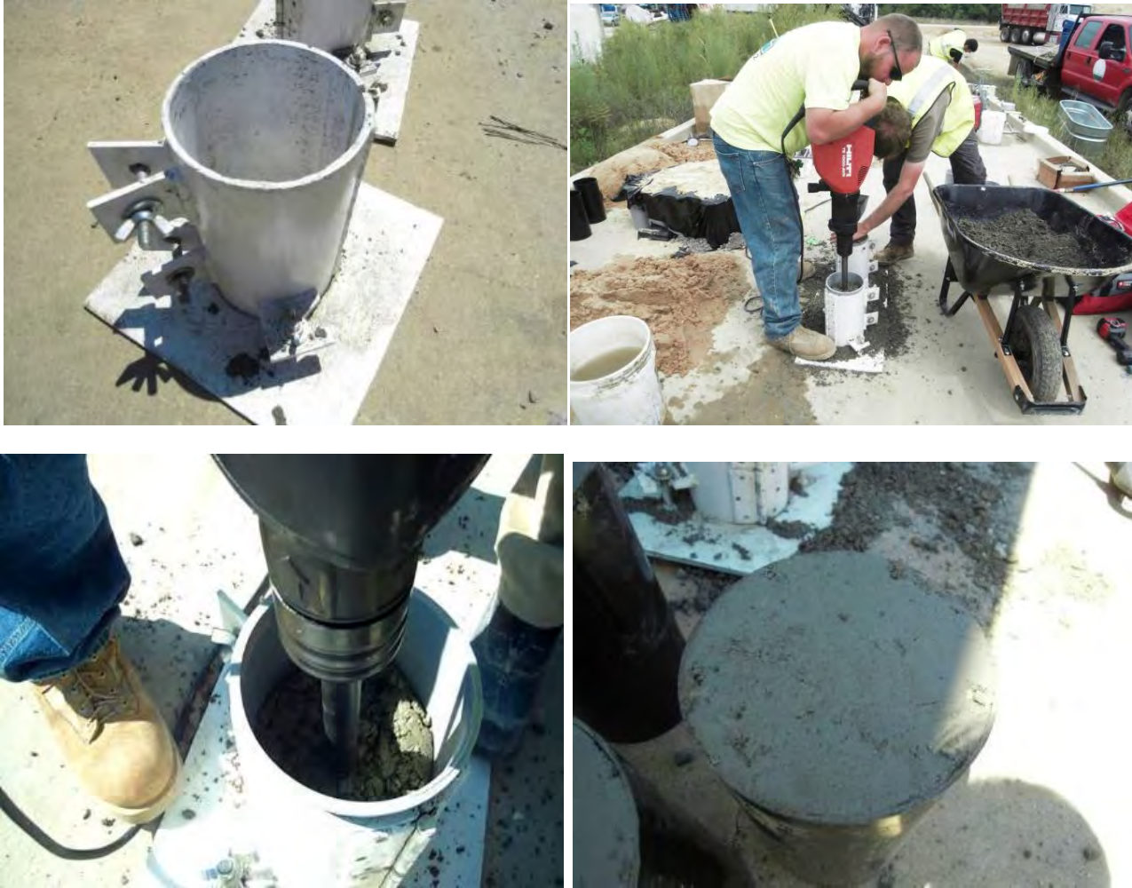
Figure 20- Sampling of concrete specimens
