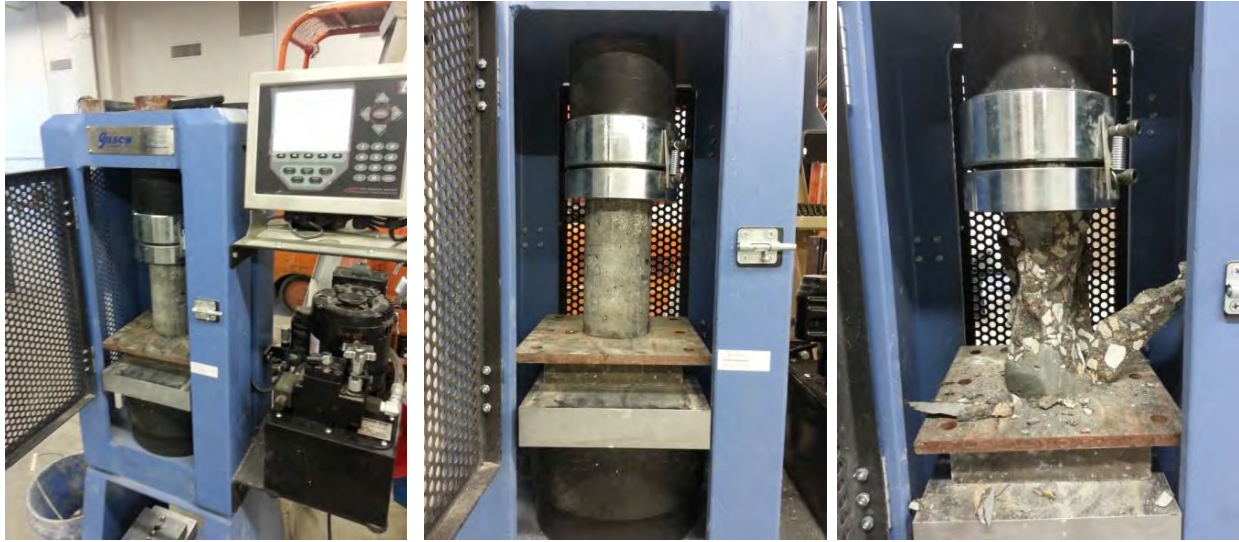
Figure 7- Compressive Strength test
