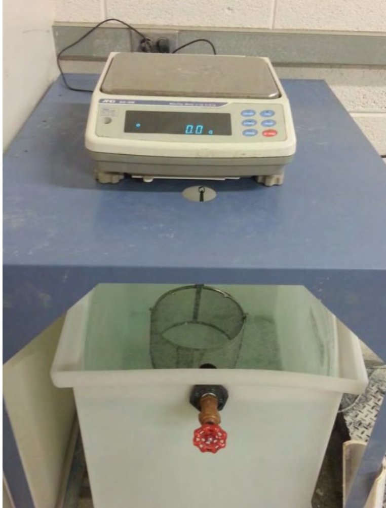
Figure 15- The apparatus used for measuring permeable voids in concrete
