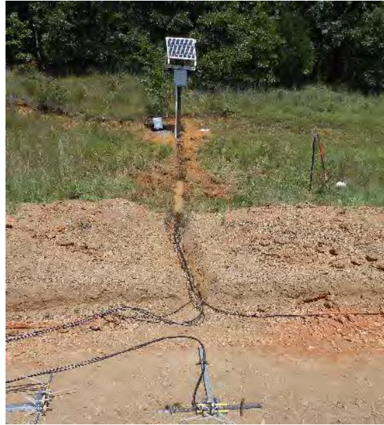
Figure 30: Tower with two installed vibrating wire gages Figure 31: Installed DAQ system powered by solar panel
