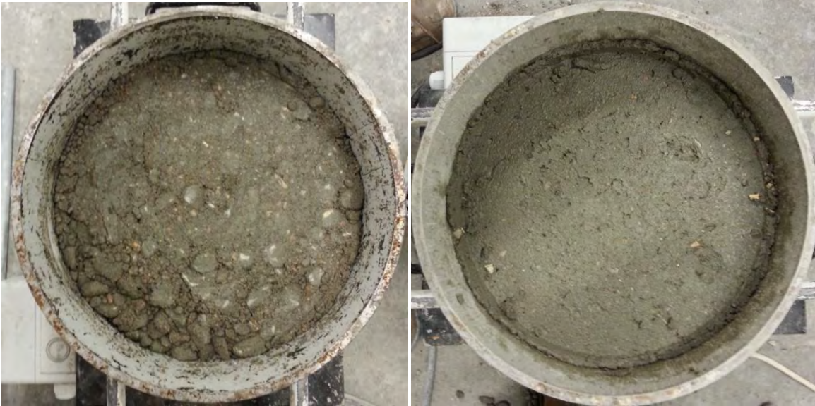
Figure 5- Concrete surface after Vebe test, left) dry RCC with Vebe >90 sec, right) RCC with adequate consistency with Vebe=45 sec
