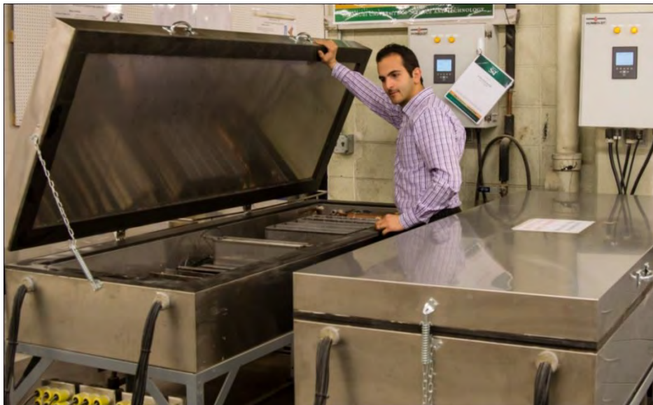
Figure 13- Freeze-thaw chamber according to ASTM C666, procedure A
