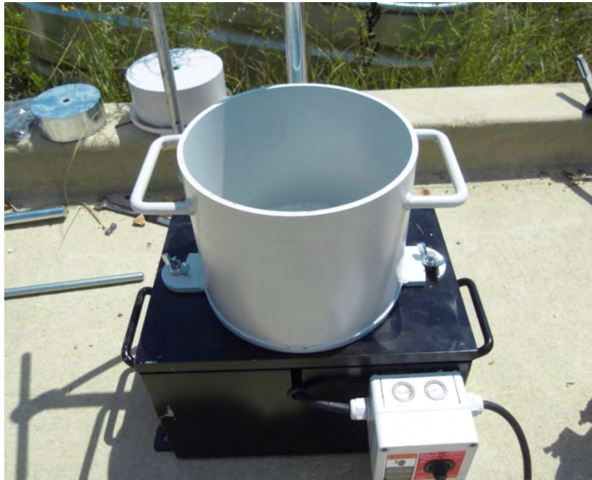
Figure 4- Vebe test Apparatus for evaluating consistency of fresh RCC
