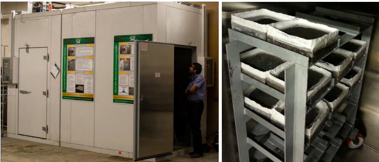
Figure 14- Chamber used for Deicing salt-scaling resistance test
